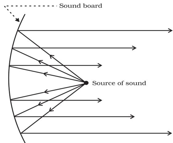
Fig. 11.13: Sound board used in a big hall.
